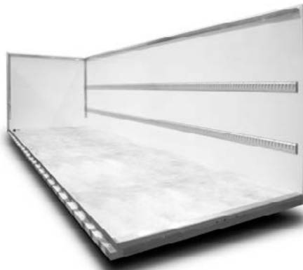
Montage von Isolierkoffer und Detail von Bodenplatte Unfinished box ARCAL FRC and detail view on the floor panel
